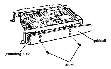
2. Remove the four screws securing the mounting frames to the hard disk drive. There are two screws securing each frame, as shown below.
